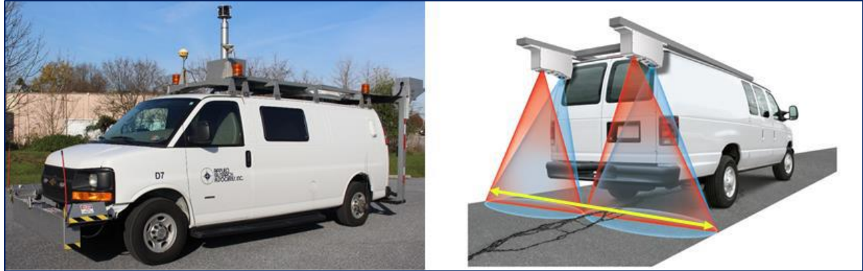
Figure 3. ARA's Laser Crack Measurement System.
