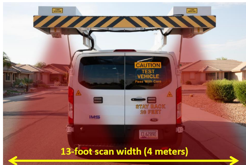
Figure 5 - RST Equipped with the 3D LCMS-2 Camera
