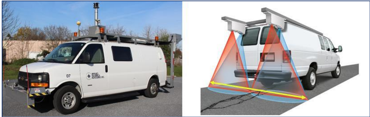
Figure 3. ARA's laser crack measurement system.
