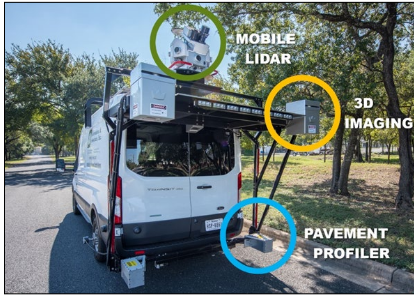
Figure 5: G&AI’s PathRunner pavement data collection system.
