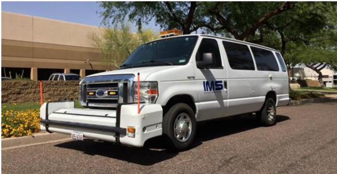
Figure 3 – Laser Road Surface Tester (RST)
