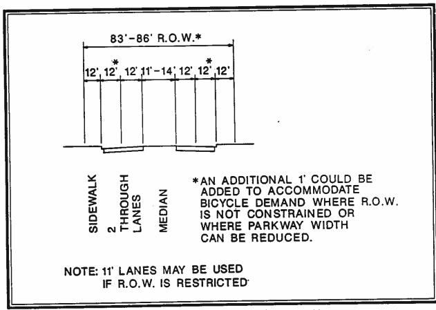
Figure 4.1A Desirable Urban SRA Cross-Section Without HOV Lanes
