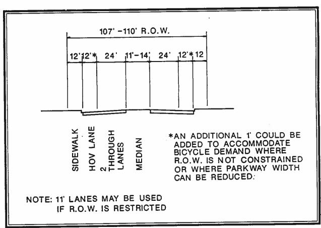
Figure 4.18 Desirable Urban SRA Cross-Section With HOV Lanes
