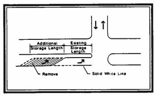
Figure 4.5 Increased Storage Capacity
