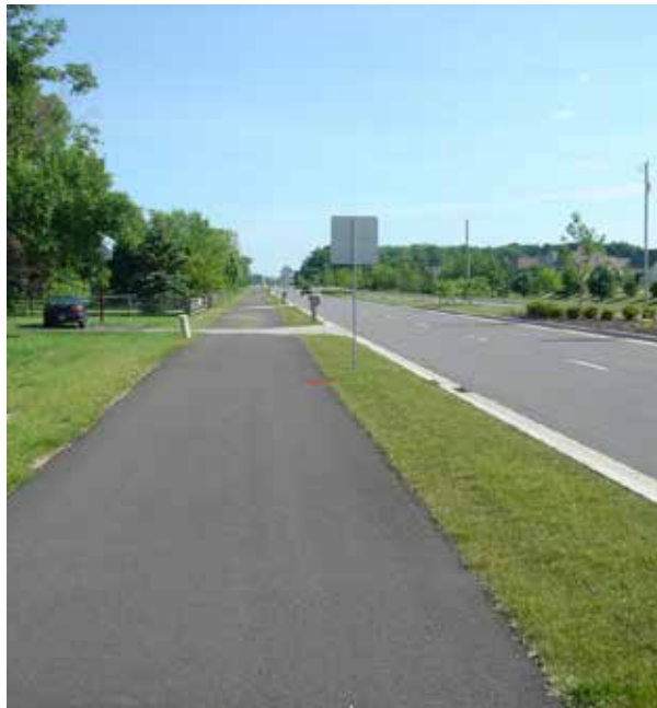
Figure 76. Off-street sidepaths are typically 10' or wider.
