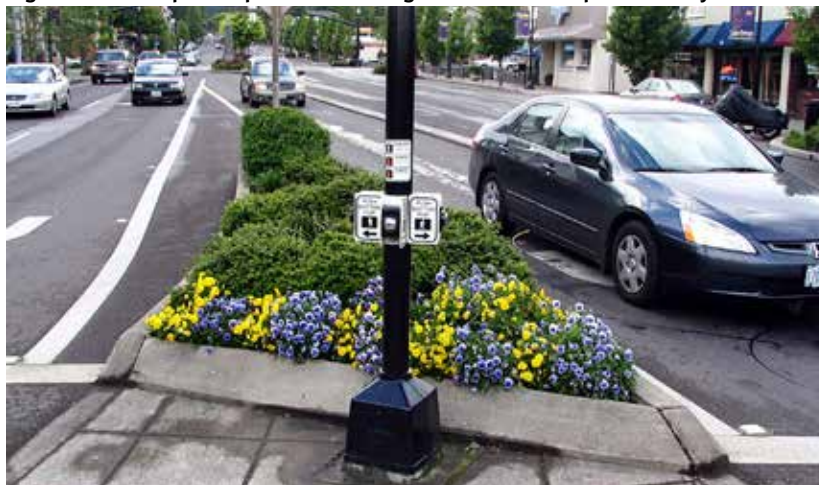
Figure 48. Examples of pedestrian refuge islands that improve safety
