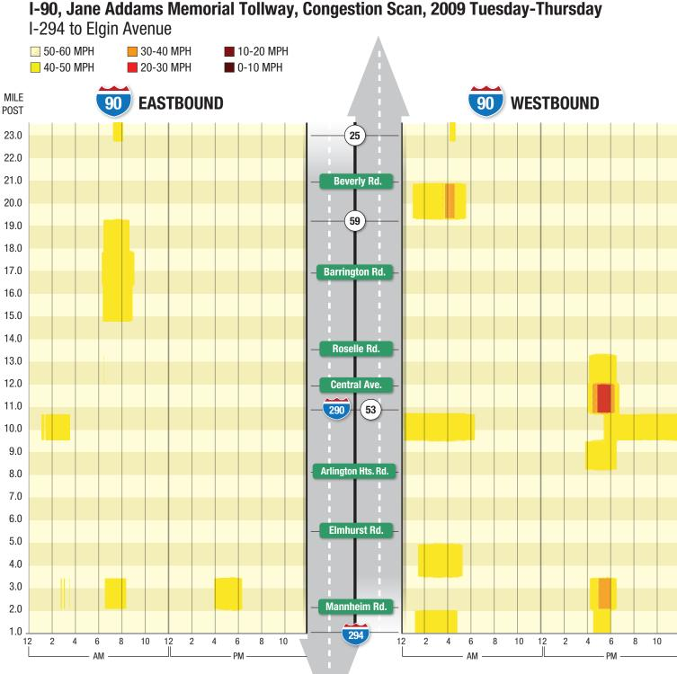
Note: Average speed is shown as a function of time of day (the horizontal x-axis) and location (the vertical y-axis).
