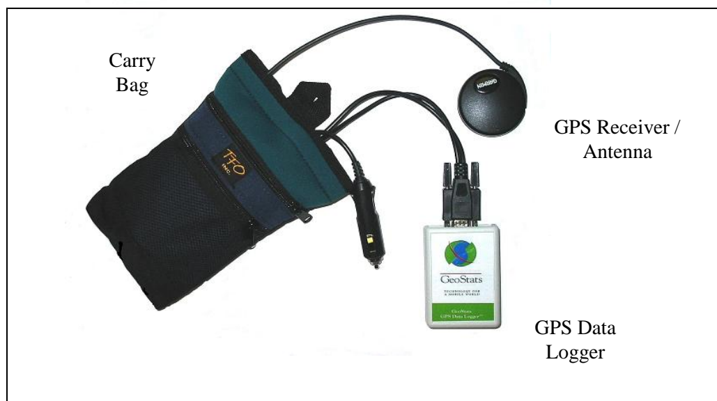
FIGURE 1: THE GEOSTATS IN-VEHICLE GEOLOGGER
