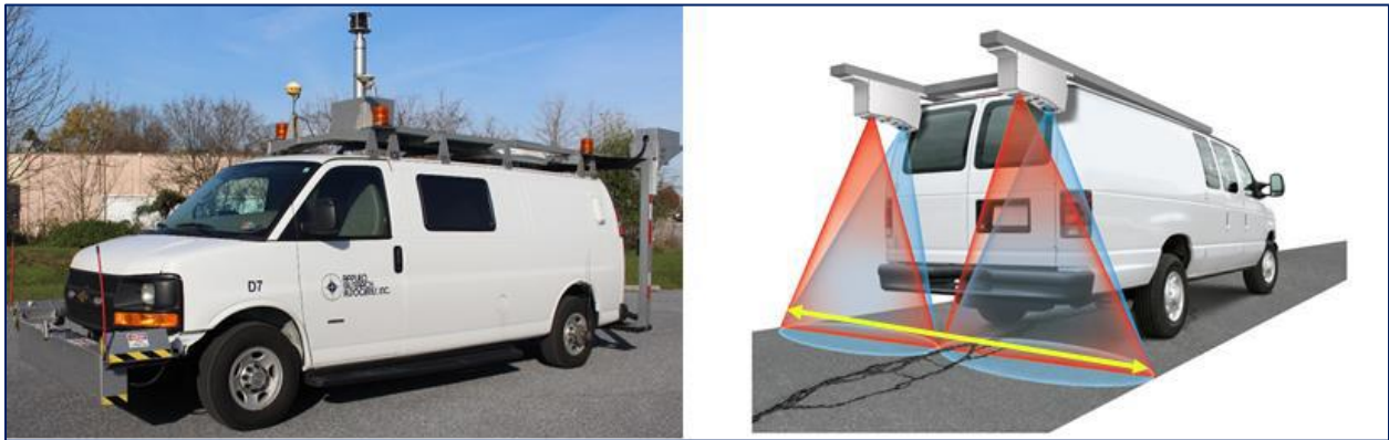
Figure 3. ARA's Laser Crack Measurement System.
