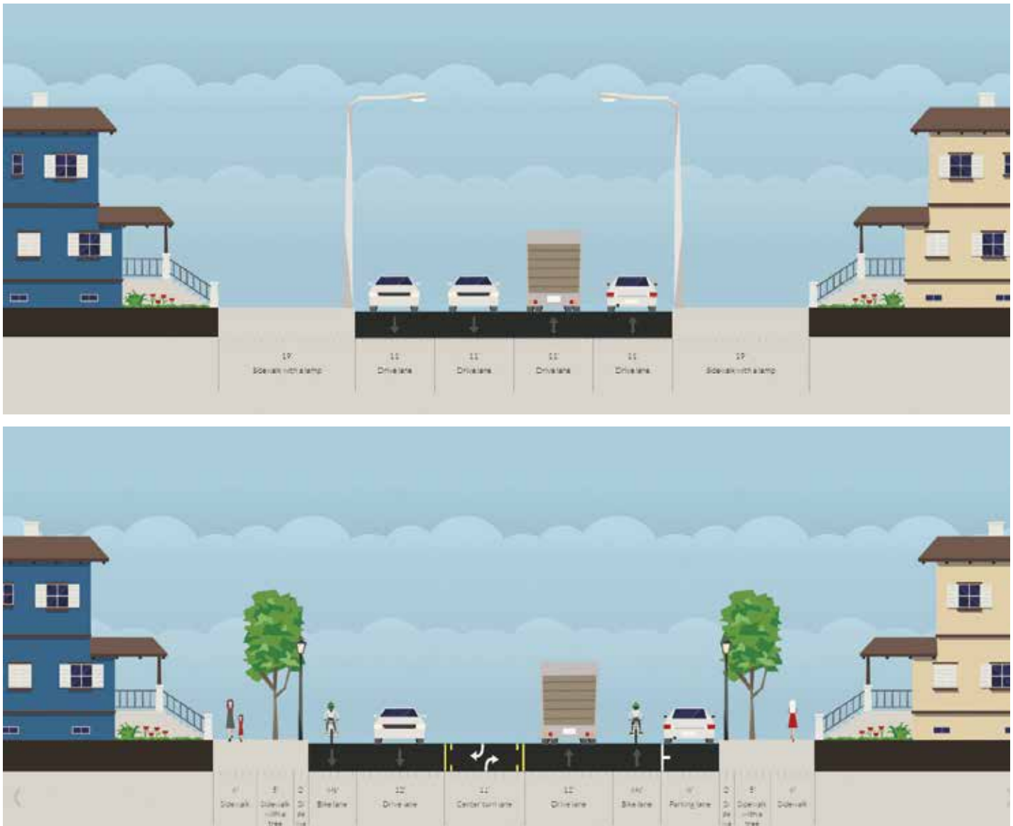
Figure 3.11. Existing and proposed street cross section, Jackson Street to Park Avenue
