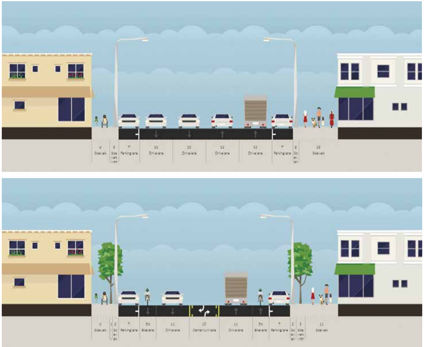
Figure 3.10. Existing and proposed street cross section, Robert McClory Bike Path to Jackson Street
