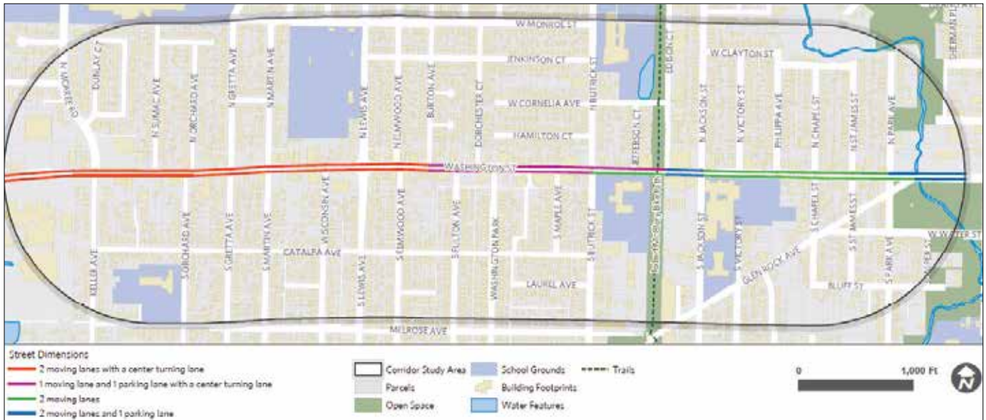
Figure 3.8. Existing lane structure
