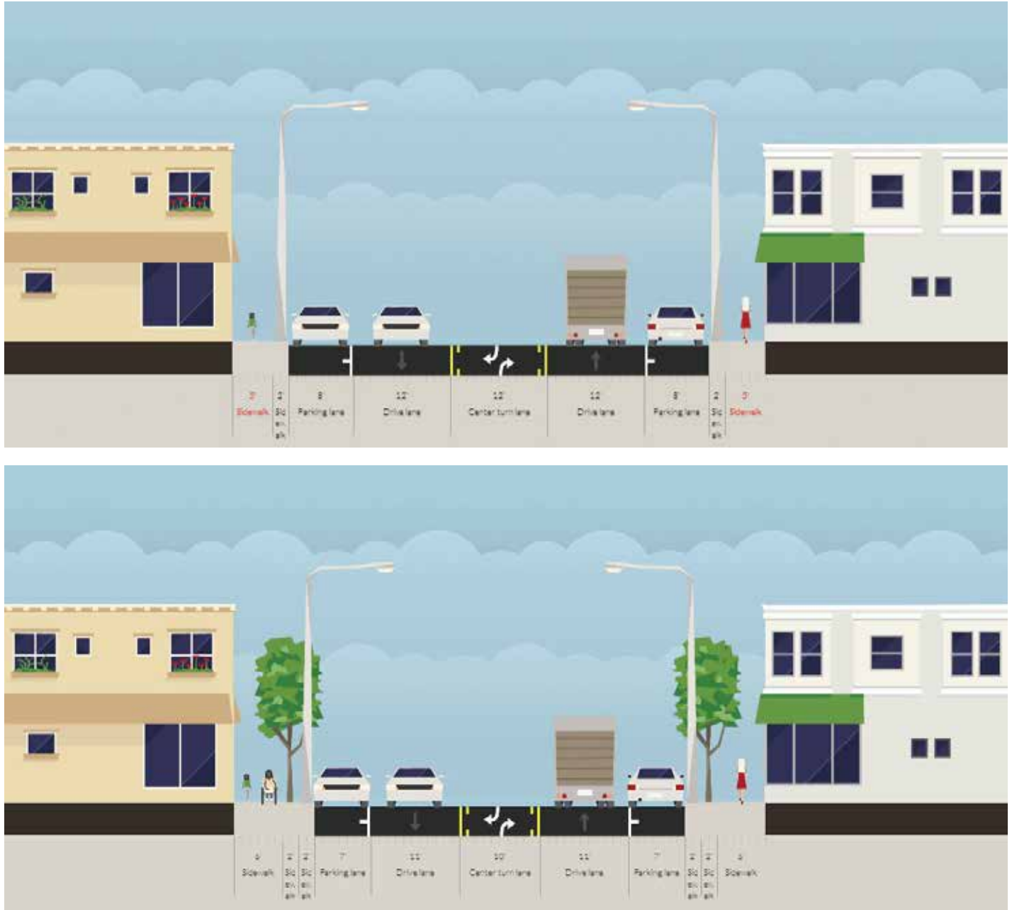
Figure 3.3. Existing and proposed street cross section between Burton Avenue and Robert McClory Bike Path
