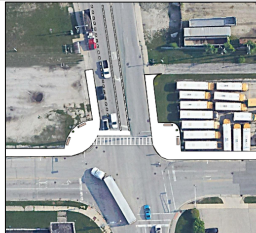
Figure 4-12. Concrete Catchment Areas on North Side of Intersection
