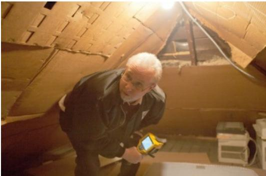
House Detectives: Michael Ruehle, a BPI energy analyst, in an attic crawl space of the Lewis home in Oak Park. Ruehle uses thermal imaging technology to determine air leaks.
