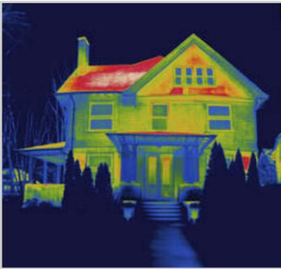
Infrared photos show where buildings lose energy as a result of poor insulation and drafts. Dark colors indicate cold spots, and a well-insulated house will look cold on a cold night because it won't be conducting heat to the outside. | Supplied Photo
