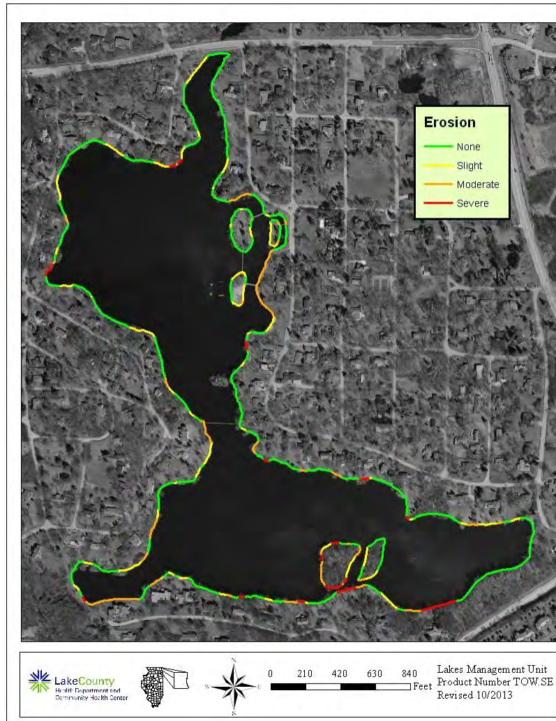
Figure 103. Tower Lake 2013 shoreline erosion condition.
