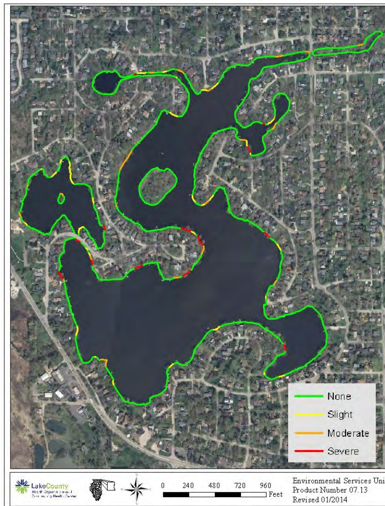
Figure 61. Island Lake 2013 shoreline erosion condition.
