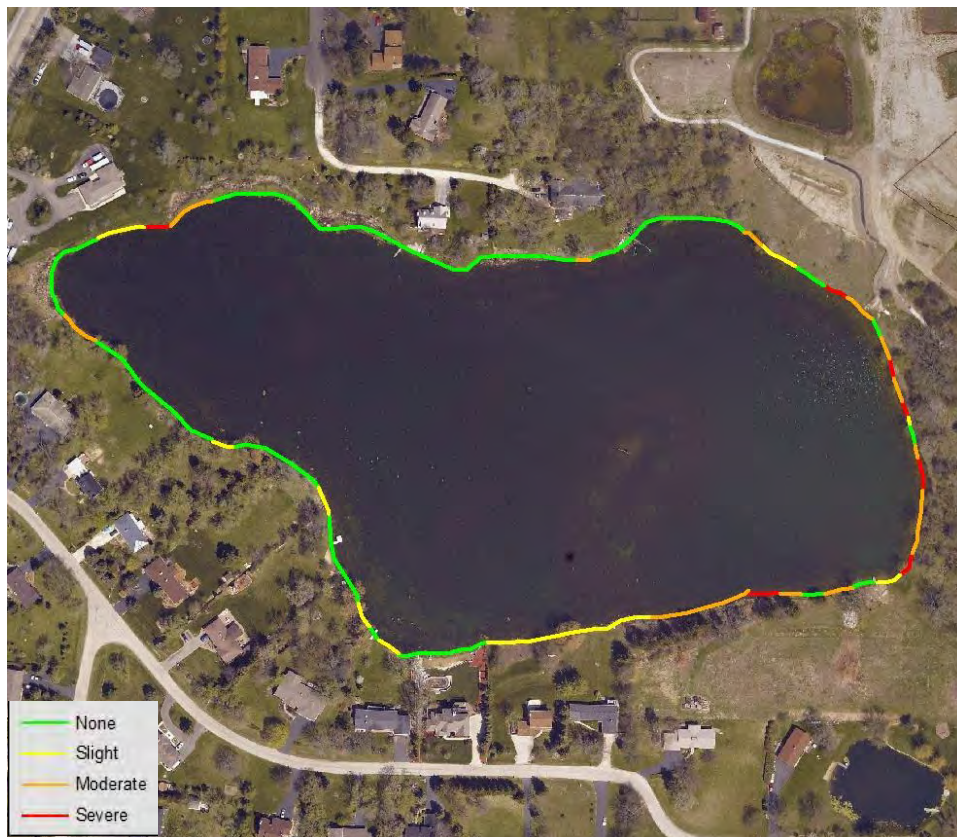
Figure 96. Lake Fairview 2013 shoreline erosion condition.
