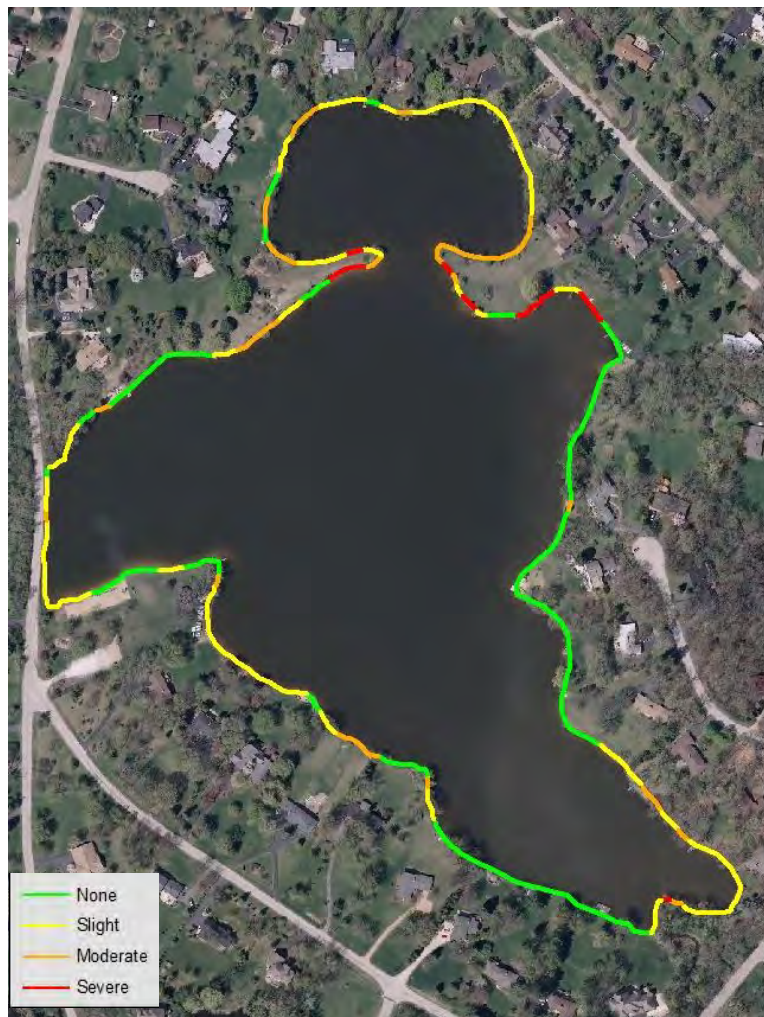
Figure 89. Timber Lake 2013 shoreline erosion.
