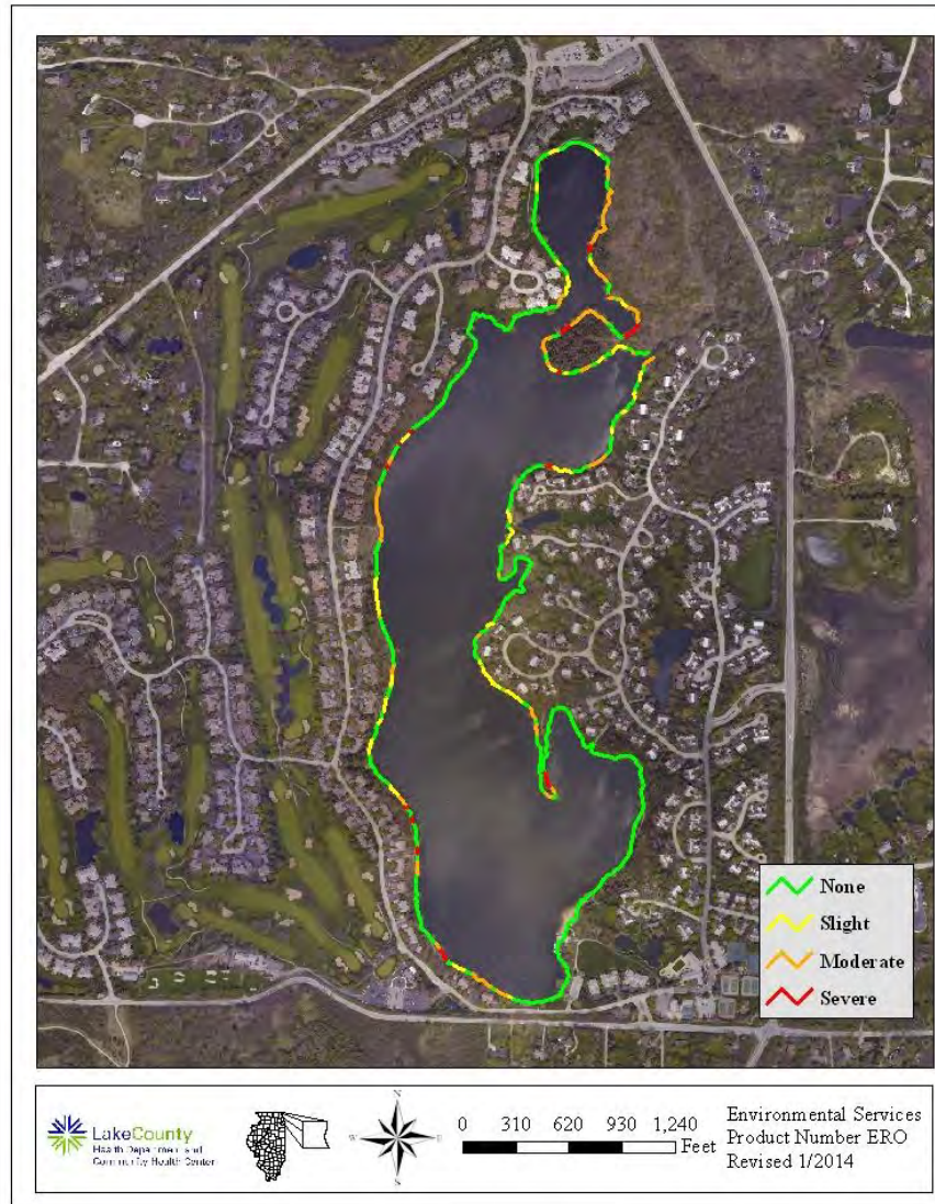
Figure 110. Lake Barrington 2013 shoreline erosion condition.
