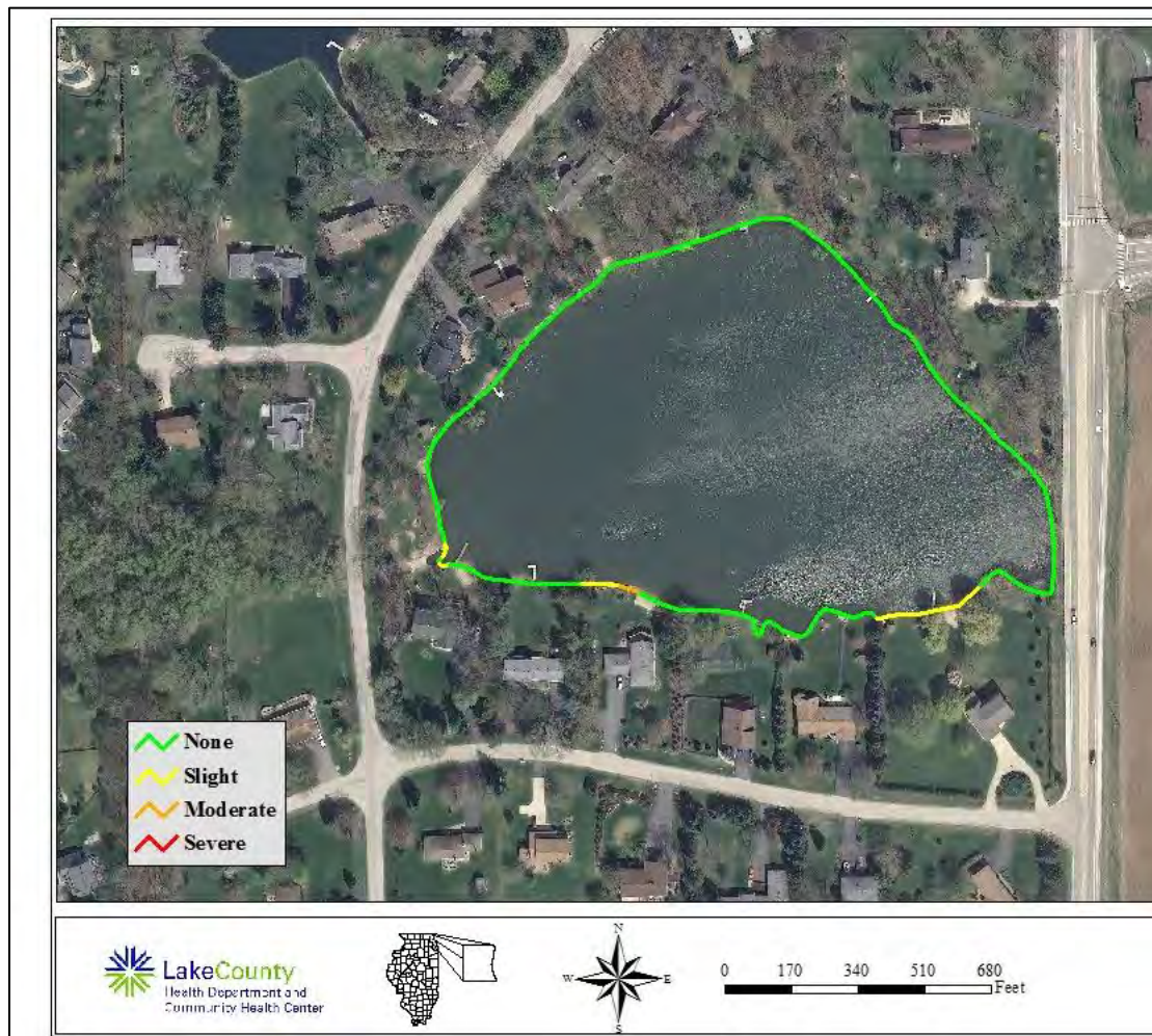
Figure 54. Woodland Lake 2013 shoreline erosion condition.
