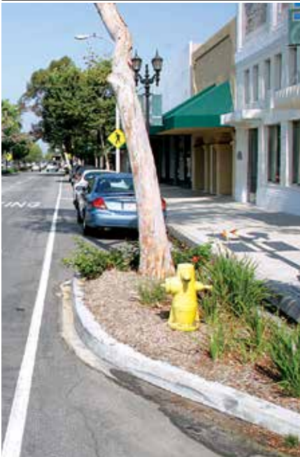
Figure 3.13. Examples of street trees in curb extensions
