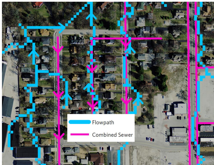
Figure 14. Example of sewers and surface flow in different directions
