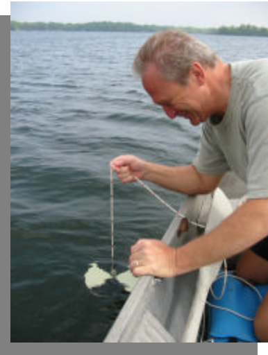
Volunteer Bob Schmidt (Cedar Lake, Lake County) uses a Secchi disk to measure water transparency.
