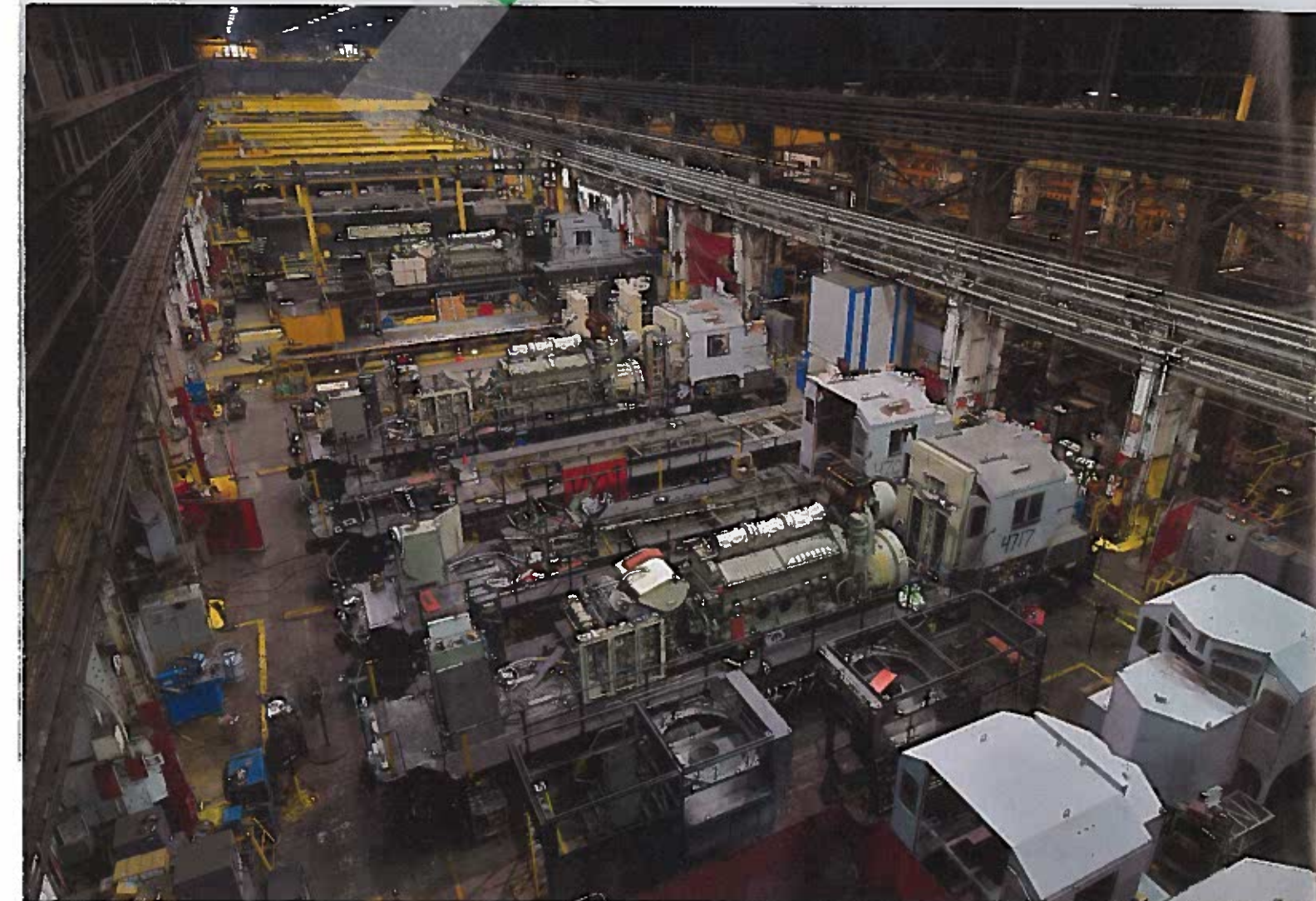
This view shows the portion of Juniata Shop in Altoona, Pa., workers call "Motherland," where locomotive assembly begins. Several GP33ECOs are in various phases. NS built all of its GP33ECOs in this shop, delivering them in 2015. Norfolk Southern: Casey Thomason
