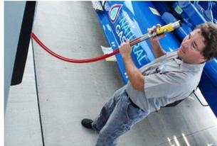
A CNG hose end has a small lever that must be turned to lock the coupling with the vehicle tank. Another difference is a 30-second limit on the time between activating the pump and starting to fuel. Diesem said that time limit is intended to prevent gas theft.
